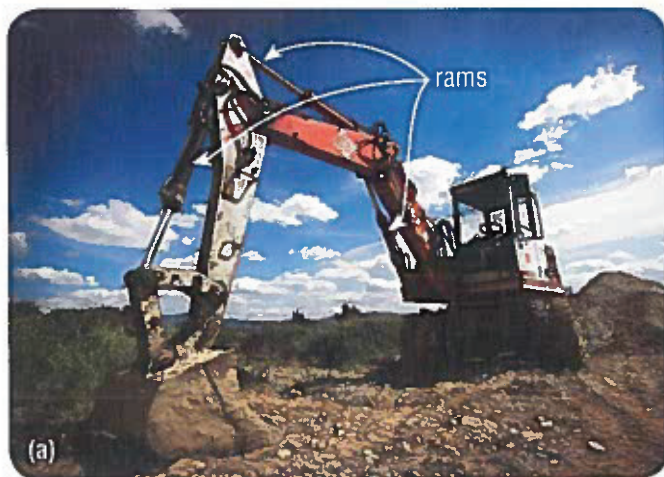
Figure 1 (a) Hydraulic rams allow this single worker to do the work of many people. (b) The rams work by forcing fluid into either side of the piston, allowing powerful and precise movement in both directions.
