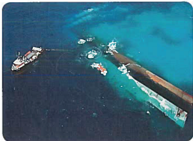
Figure 1 The buoyancy of water was used to roll the Spiegel Grove onto its side so that it would be totally submerged.
