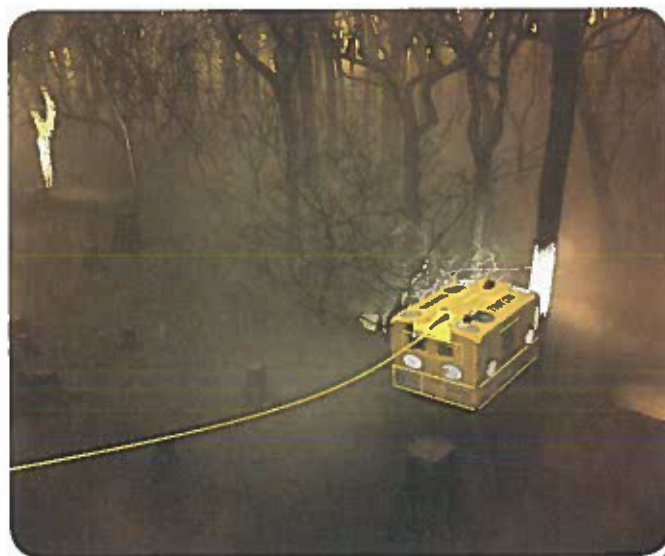
Figure 2 The Sawfish uses the buoyancy of water to manoeuvre, handle cut trees, and bring them to the surface.
