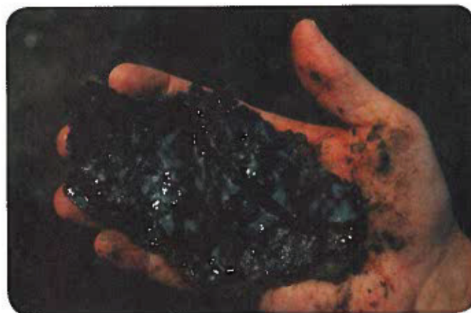
Figure 2 About 2 tonnes of oil sand are required to produce 1 barrel of oil.
