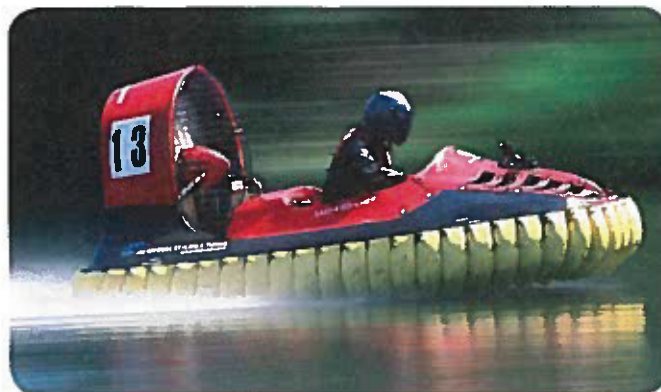
Figure 3 A hovercraft is a pneumatic system.
