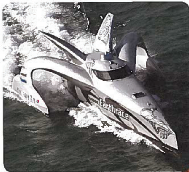
Figure 2 Earthrace 's streamlined, wave-piercing design allows it to travel smoothly through the water as well as on it.
