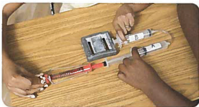
Figure 2 Slowly push on the force meter while taking the measurement.
