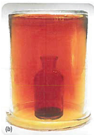
Figure 2 The brown bromine gas in the small bottle slowly moves out of the bottle (a) and fills the large container (b).
