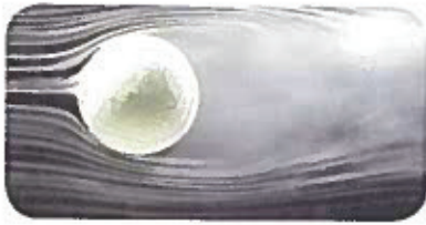
Figure 10 Wind tunnels and smoke trails can be used to investigate patterns of fluid flow around objects like this tennis ball.
