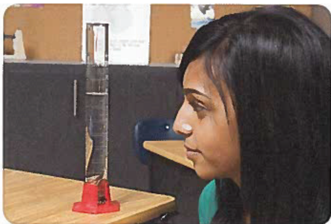
Figure 1 Remember to read the graduated cylinder at eye level.
