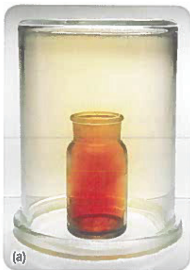
Figure 2 The brown bromine gas in the small bottle slowly moves out of the bottle (a) and fills the large container (b).
